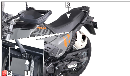
(1) Helmet holder hook (2) Wire helmet set (3) Seat
