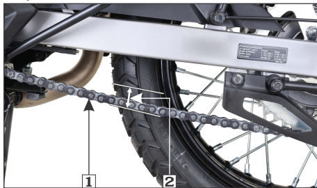
(1) Drive chain (2) Drive chain slack: 30–35 mm
