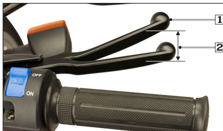
(1) Front brake lever (2) Free play 10–20 mm
