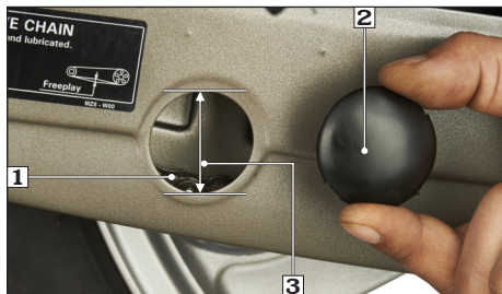
(1) Drive chain (2) Hole cap (3) Drive chain slack 25 mm
